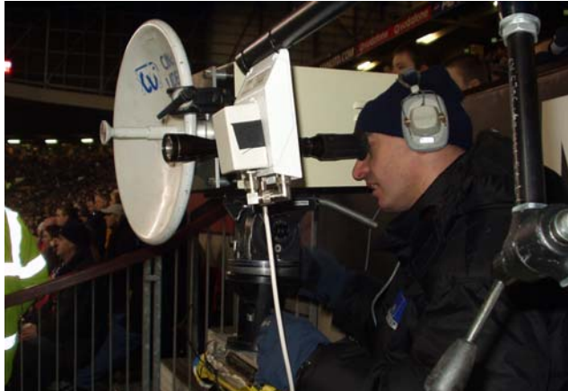
Figure 5 - Typical analogue system showing the very directional antenna and telescope used to align it with the transmitter
