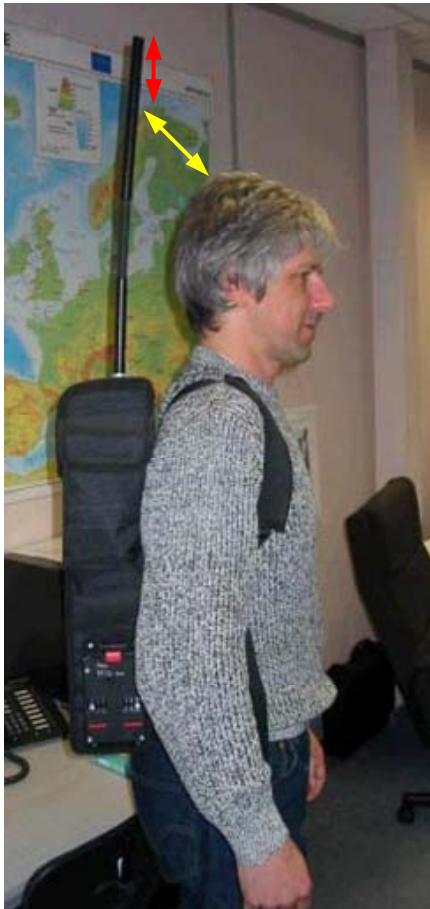
Figure 4 - Rucksack mounted system showing long antenna with radiating section well above the cameraman's head.
